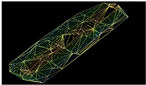
70. Scan Radius: Scan radius will direct the program to pick points falling with in such radius to generate TIN surface. If the points are away from the scan radius they would not join the adjacent surface and kept isolated.
