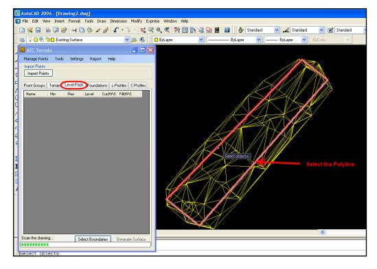
88. The Boundary lines (Selected closed polylines) shall be listed in the Data Grid with captured data from the AutoCAD, like minimum and maximum levels with naming as B1, b2 B3 and so on.. as boundaries. These boundaries can be renamed as the user wishes them to be.
