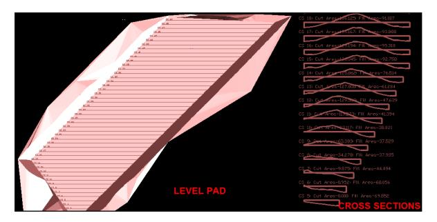
91. Level Pads file (containing the final surface points) will be saved in the Input folder. A CSV file is written to the folder path containing coordinates in NEZ format. This file when plotted again would make a flat TIN surface as shown in the image below. Click on OK
