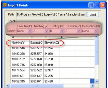
Click command button to load input file. Click on Import to load the input points file
