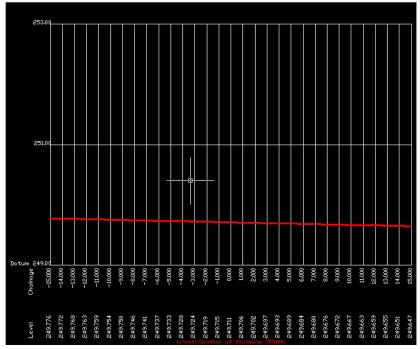
c) Level Row Spacing: Program writes/plots datum levels in graph at this spacing. For example case we have the level intervals are 249, 250, 251 and so on at 1 meter intervals. If we change this value to 2 meter intervals we will have 249, 251, 253 and so on.
