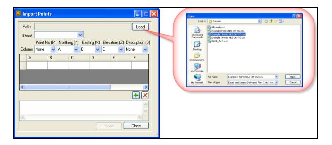
41. Map the points file as per the required format Ex: Northing(Y), Easting(X) and Elevation (Z) format in the column as shown in the below image.
