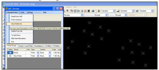
Additional points which are created manually. Two Point files will be combined and will be saved as user defined name, such as, **Contour Points File\_NEZD\_YXZD\_1** to the file location indicated by the user. The newly Saved as file with points looks as under
