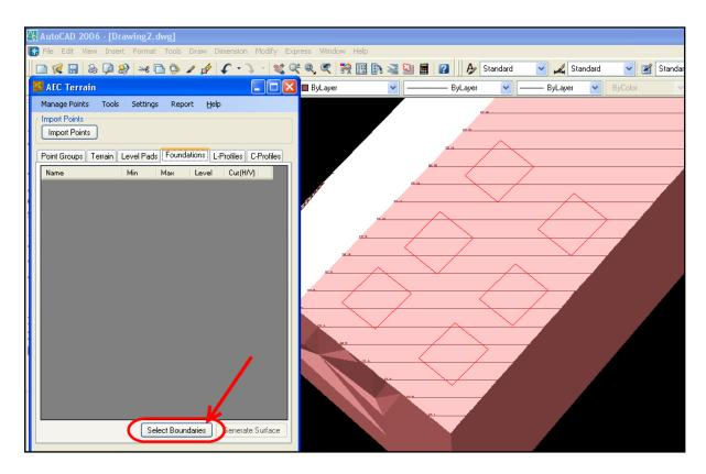
95. Select foundation Boundary Polyline(s), Then Click OK to select the polylines in the AutoCAD drawing.
