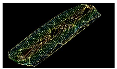
85. Scan Radius: Scan radius will direct the program to pick points falling with in such radius to generate TIN surface. If the points are away from the scan radius they would not join the adjacent surface and kept isolated.
