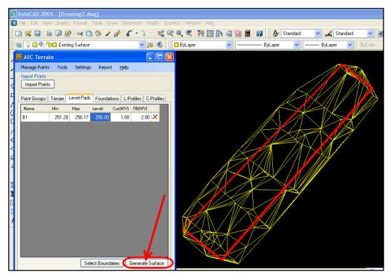
90. The program draws cross sections along on the level pad flat surface and slopes with chainage marking for computations checks. Indicate a point on the AutoCAD to draw these Cross-sections when prompted by the program.
