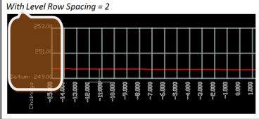
d) Min. Space B/W CS Graphs: The Spacing between two Cross Sections. This setting plots in either X or Y directions at the specified spacing.
