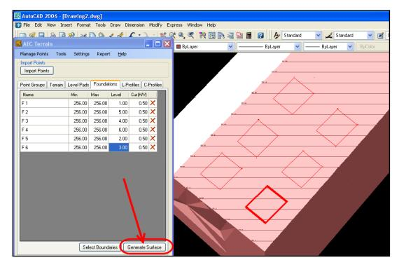
96. Set the levels for the foundation as desired. Then click on Generate Surface. Interference of the adjacent footings shall be taken care by the program.
