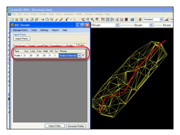
105. Save the Output Cross section file at desired project folder location. The file contains the coordinates of all the generated from the terrain.
